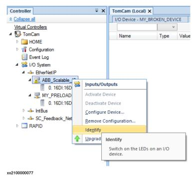
3 The PWR (Power), MS (Module status) and NS (Network Status) LED of the physical base I/O device flashes to identify the I/O device in the controller.
